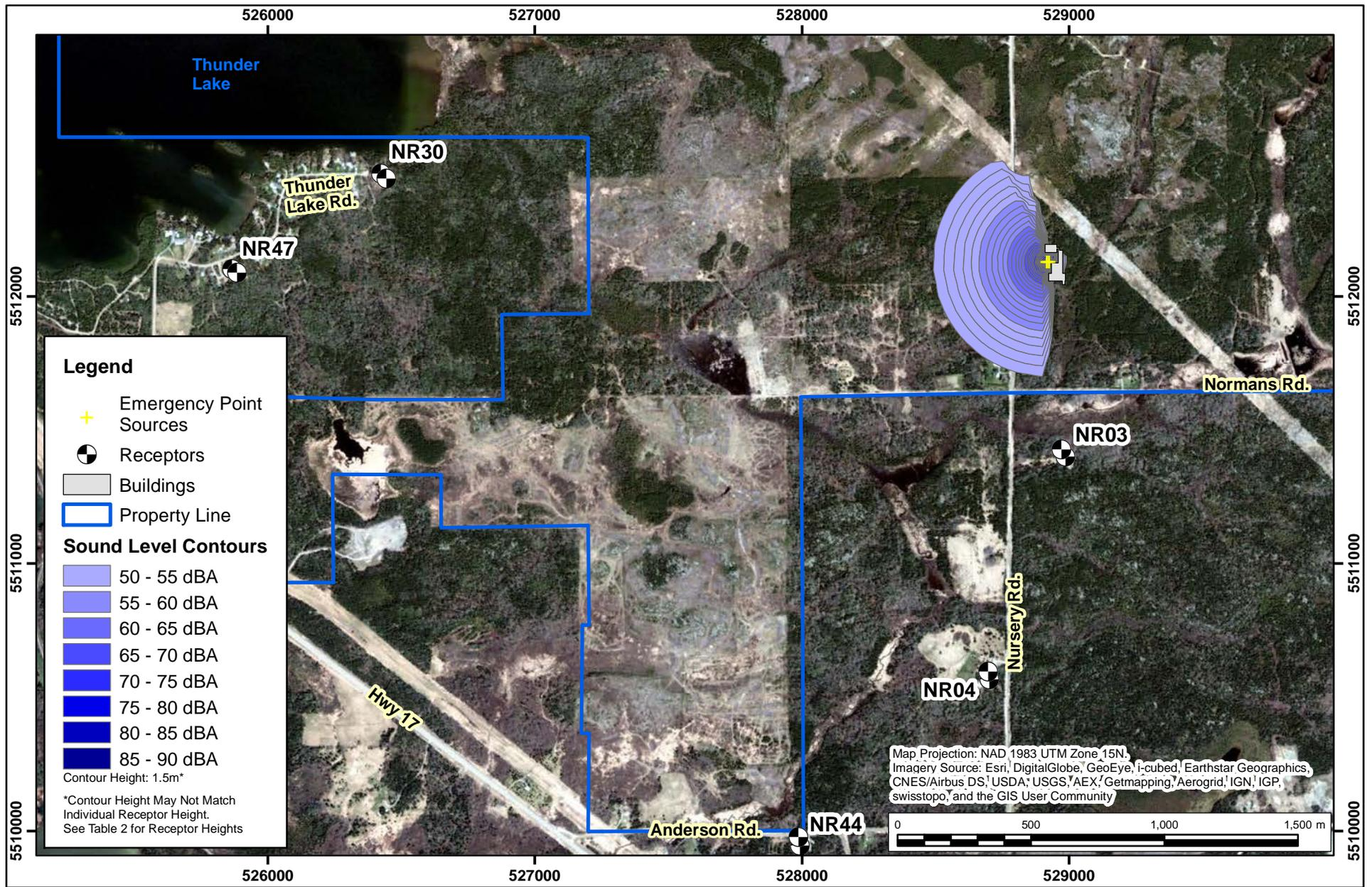
Predicted Sound Level Contours for Emergency Source Testing
